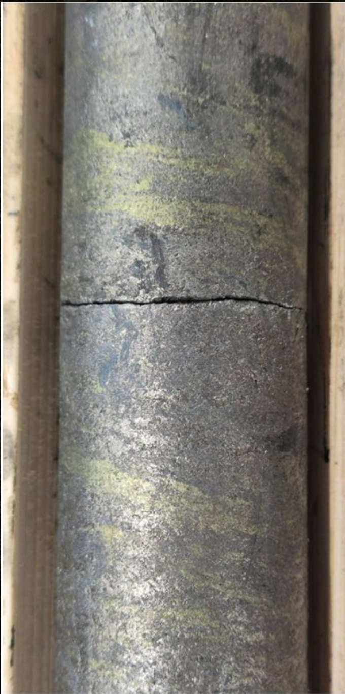
Photo 1: Massive pyrrhotite with about 10% chalcopyrite in regular bands at 85 degrees core angle . Center of photo was taken at 243.75m in hole CUP26-06
