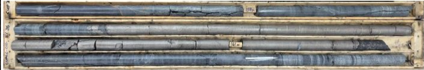
Figure 1: Photograph of the 2.45 meters thick chalcopyrite-bearing massive sulphide horizon 80-85 degrees to core axis located at the base of a sulphide bearing (blebs and disseminations) olivine pyroxenite. From 159.1 to 161.55 meters in hole CUP26-010.
